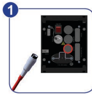
Fig. 22: Connecting the actuator cable – step 1
