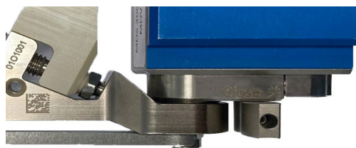
Fig. 35: Screwing tight the nozzle fixation nut
