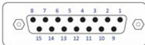
Fig. 62: PLC Interface: 15-pin, Sub-D
