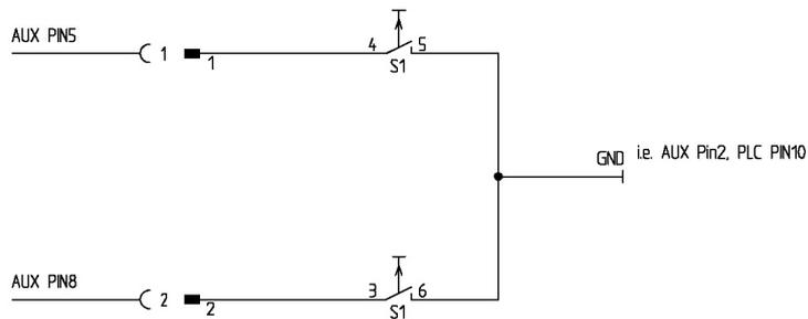
Fig. 54: Schematic of usage of select pins
