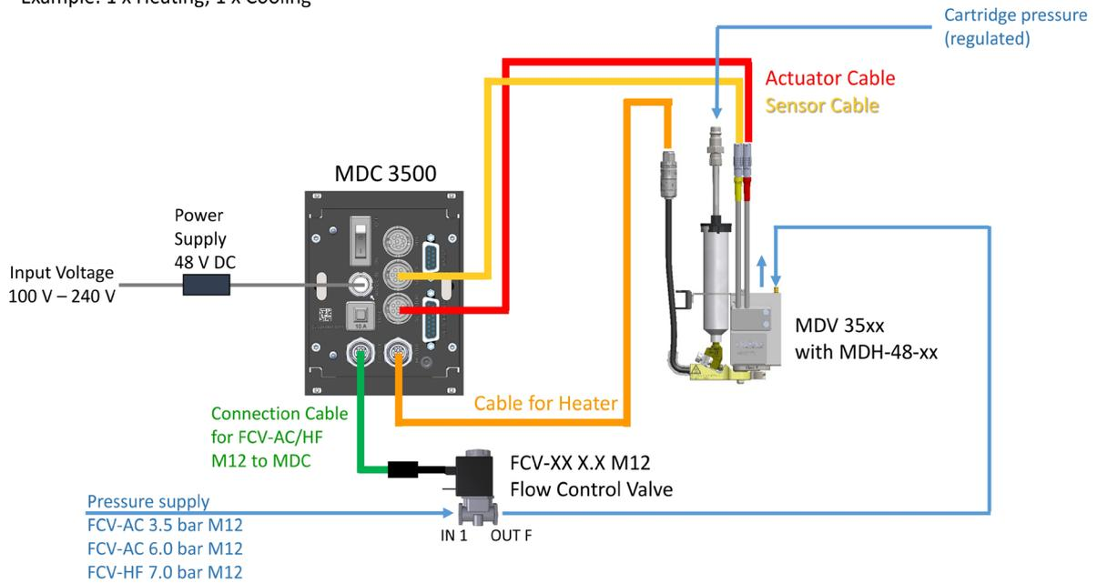
Fig. 81: Connection Diagram MDS 3580
