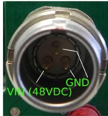
Fig. 3: Connection for power supply 48 V DC – pin functions
