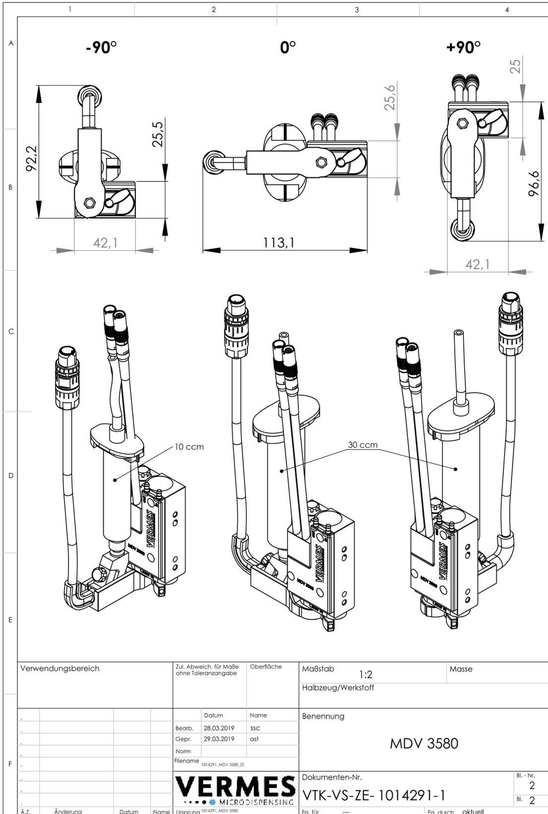
Fig. 78: Dimensional Drawing MDV 3580 positioning
