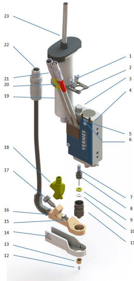
Fig. 19: Explosion view valve
