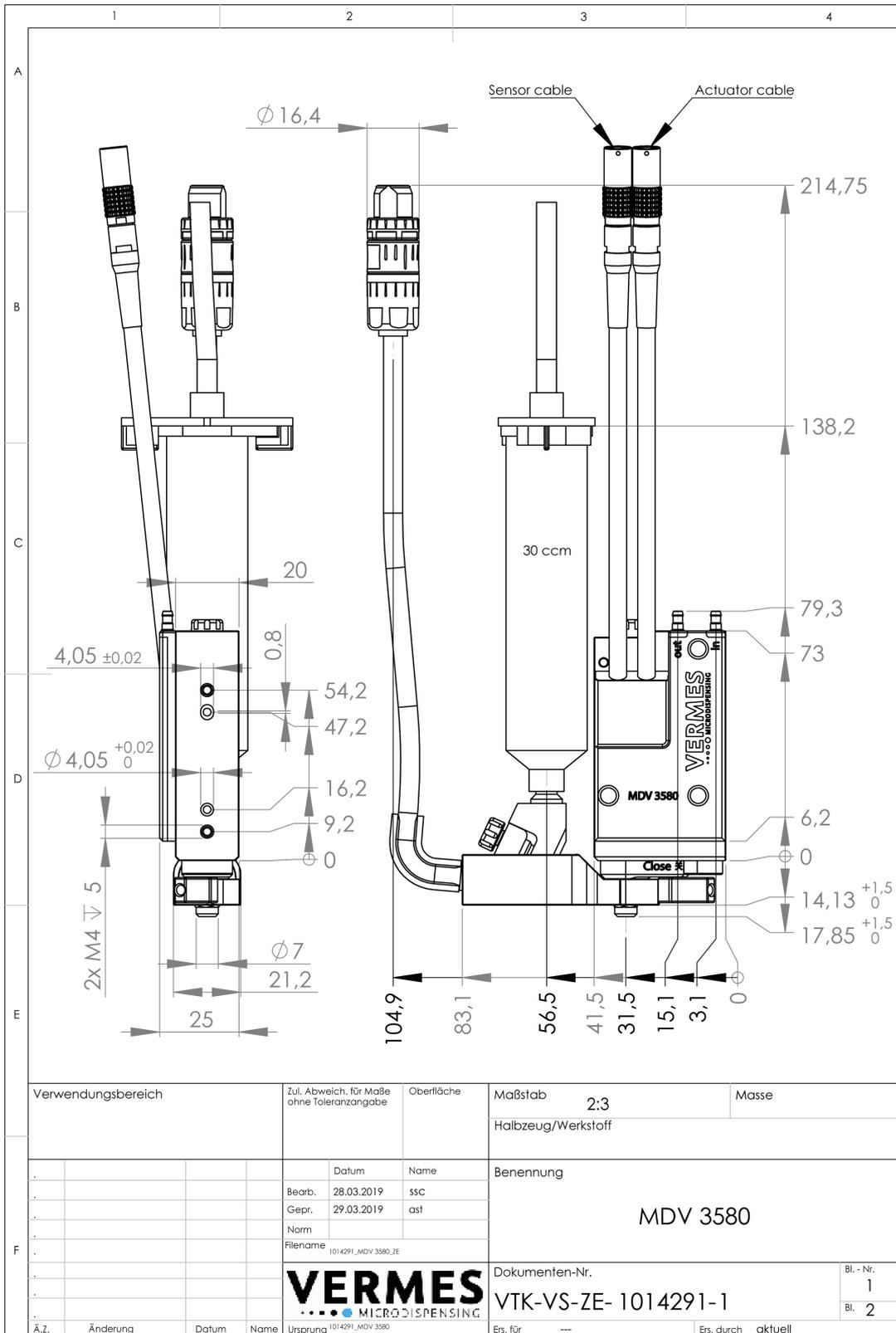
Fig. 77: Dimensional Drawing MDV 3580 front and sides
