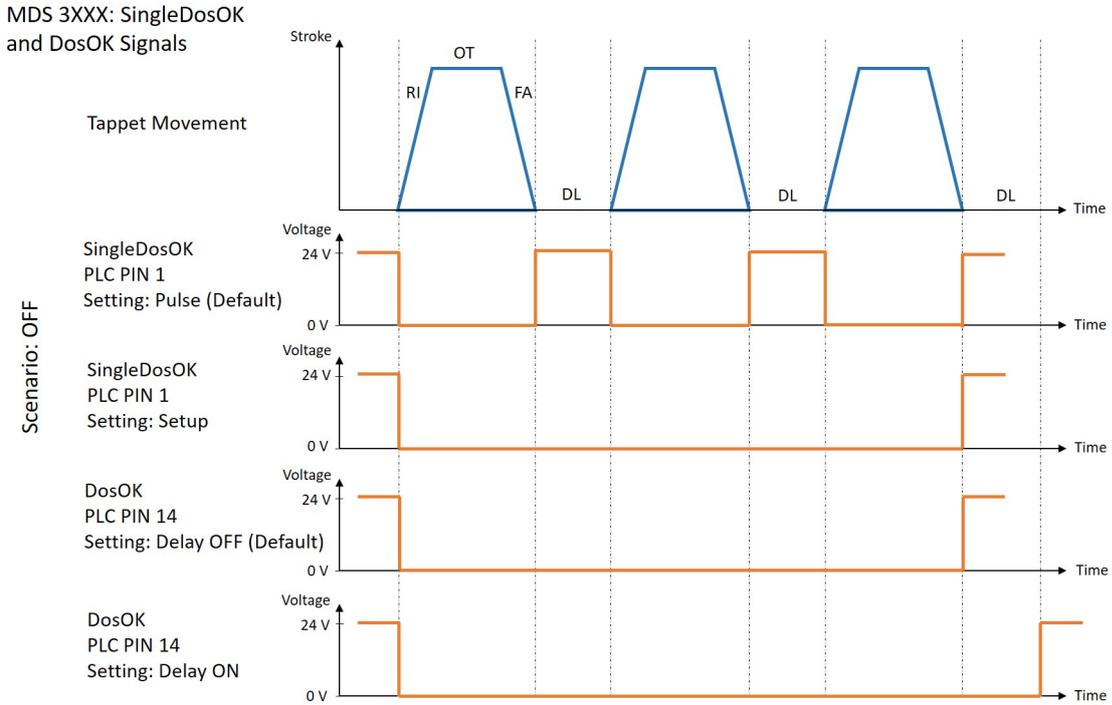
Fig. 67: PLC signals with Scenario OFF
