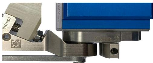
Fig. 35: Screwing tight the nozzle fixation nut
