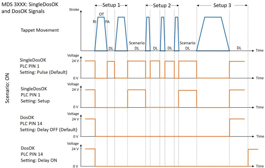
Fig. 68: PLC signals with Scenario ON
