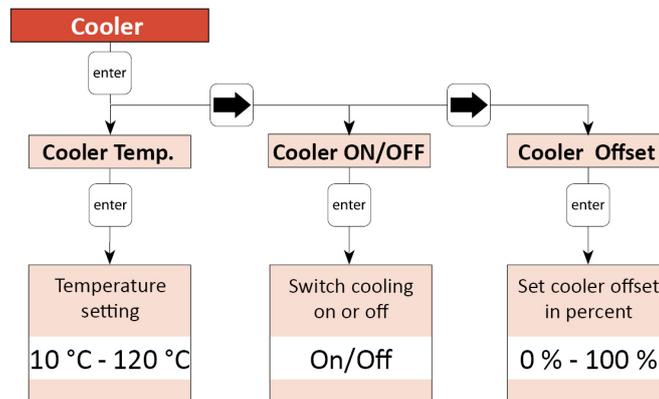
Fig. 10: Submenu "Cooler"
