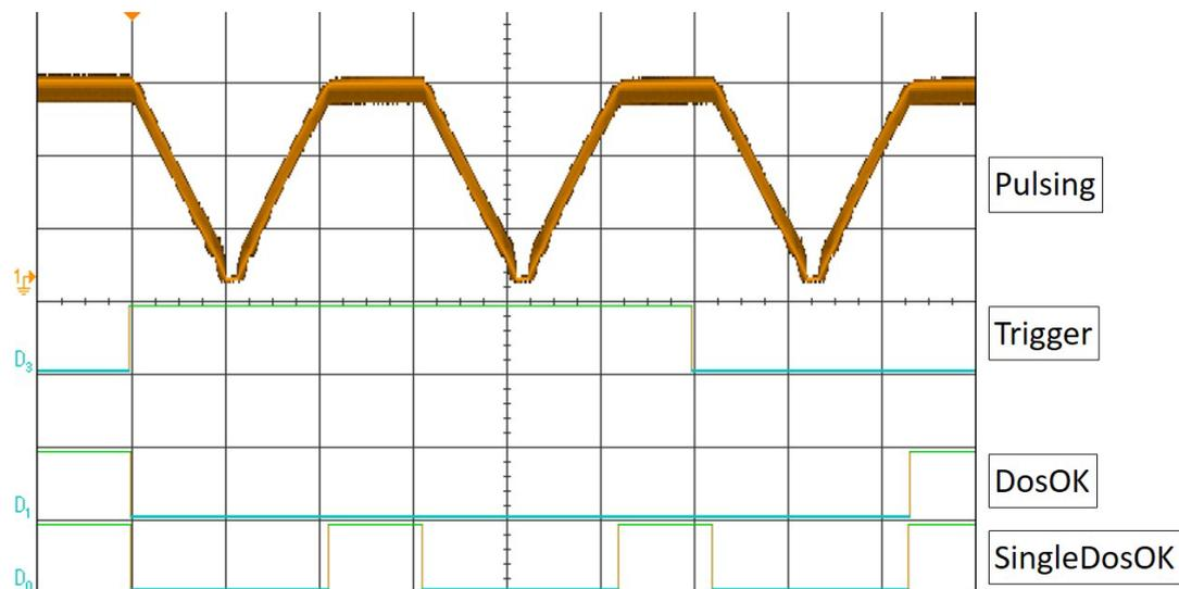
Fig. 64: Burst Mode (Example with Three Shots)
