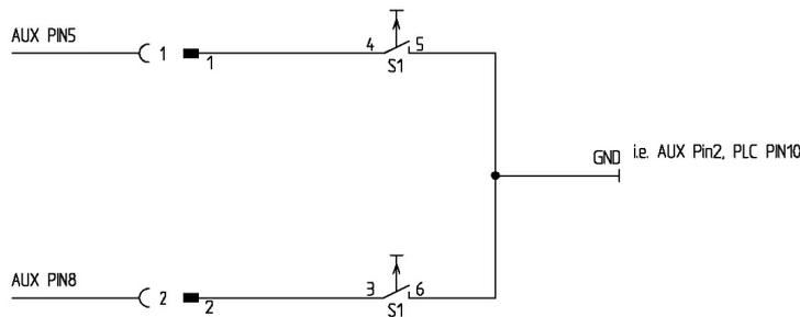
Fig. 50: Schematic of usage of select pins, example
