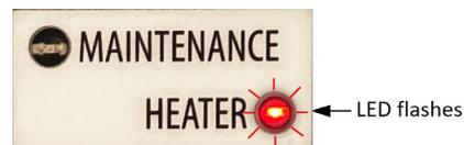
Fig. 12: Before reaching the target temperature
