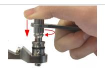
Screw the Tappet Centering Screw BY completely into the fluid box (torque 100 – 140 cN.m) with MDT 303 - Nozzle Insert Changing Tool.
