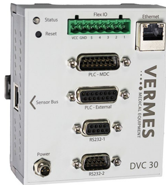
Fig. 17: DVC without any connection cables
